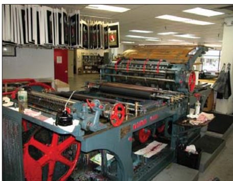
A rare Marinoni Voirin stone lithograph printing press owned by Rue Royale Fine Art and pictured in the print-maker’s Las Vegas studio. Made in Paris, the press is over 100 years old.
